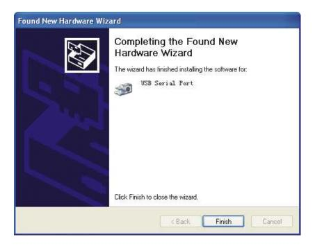
After installation, you can open Device Manager to check it there are COM ports available now, if no USB drivers have been installed previously. System default COM ports are COM 3, as illustrated below. Now, all the installation is finished.
