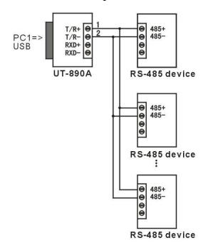
Half duplex connection between UT-890A interface converters
