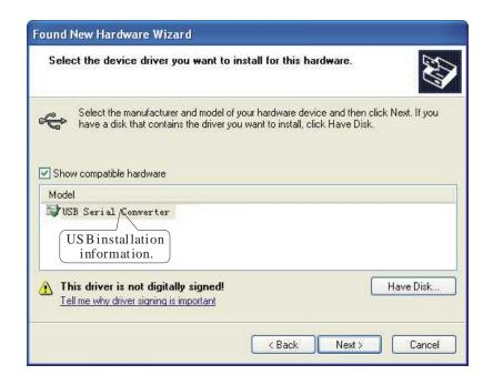
The following shows that the USB Serial Converter installation is finished, then the system wizard will detect USB Serial Port automatically.
