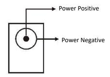
9V ±1/50mA DC power supply can be used when the serial port voltage is low
