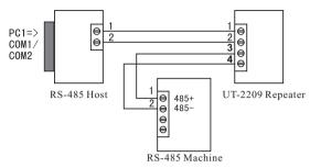
2. RS-485 point-to-multipoint 2-line half duplex relay communication
