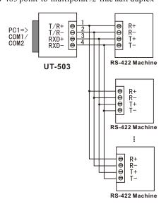
3. Half-duplex communication connections between UT-503 interfaces
