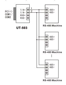
3. Half-duplex communication connections between UT-503 interfaces
