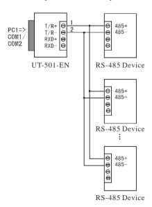
${\it 3. Half-duplex communication connections between UT-501-EN interfaces}$
