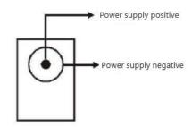
When the voltage is low, the 5-12V/20mA DC power supply
