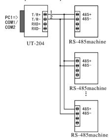
3.UT-204 half-duplex communication connect between interface converter
