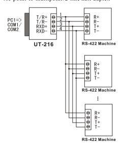
3. Half-duplex communication connections between UT-216 interfaces
