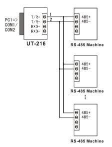
3. Half-duplex communication connections between UT-216 interfaces
