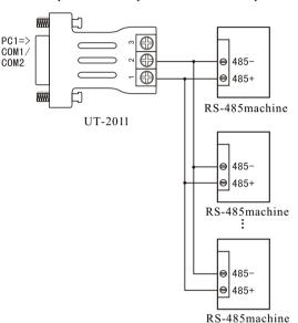
3.UT-2011 half-duplex communication connect between interface converter
