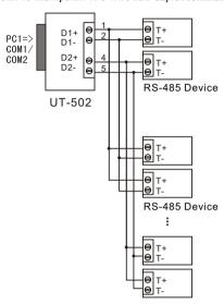
3) Any one group D1 or D2 is necessary to be connected for half-duplex communication between UT-502 interface converters
