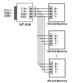
3. Half-duplex communication connections between UT-218 interfaces
