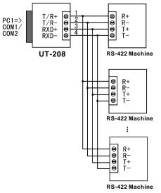
3. Half-duplex communication connections between UT-208 interfaces
