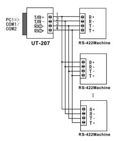
3. Half-duplex communication connections between UT-207 interfaces
