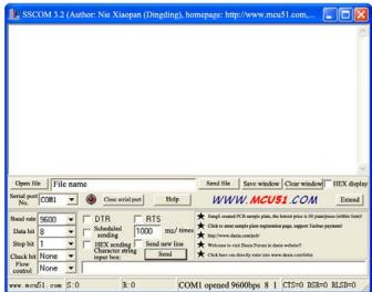
After the settings of serial port debugging software, press CFG button for 3-5 seconds and then the following interface will show (different software version will have different interfaces)
