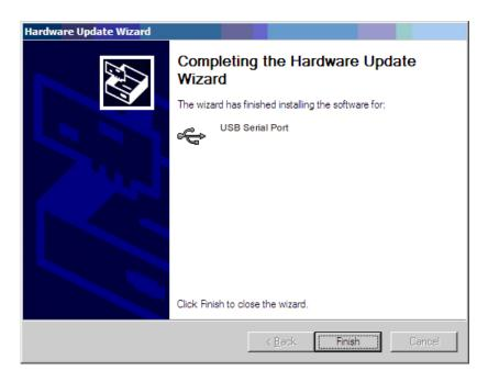
After the driver has been installed correctly please have a look at the device manager to make sure whether there is virtual COM port. If it's the first time to install the USB driver on this system then the default COM ports are COM3 and COM4 as shown in the following figure. Up to now the driver of UT-8812 has been installed successfully.
